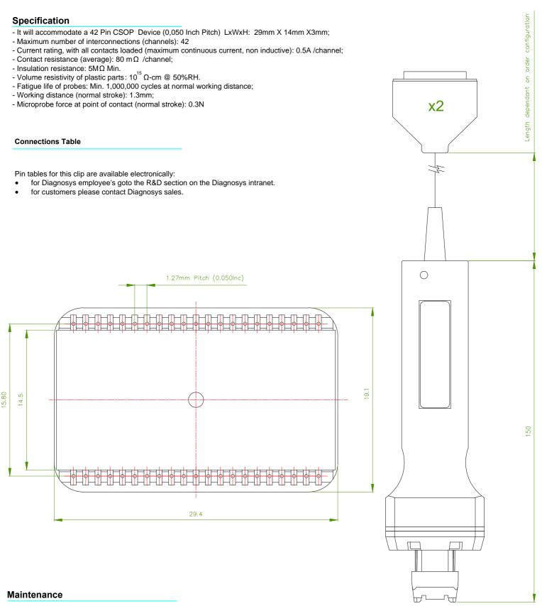
The Test Interface Head is maintenance free. The probes are self-cleaning. Immersion in water or contact between probes and any liquids should be avoided, as this could severely reduce the working life of microprobes.
