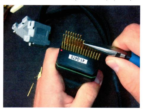
c) Pull straight up on the pin away from the UTI with the pliers.
