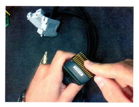
c) Then, using the end of your pliers ensure that the pin is fully seated in the receptacle.
