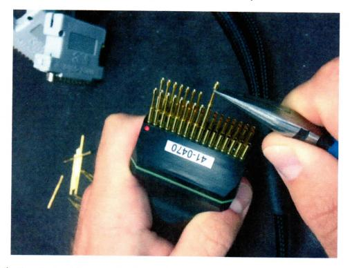
d) The pin should come out with a little effort, but be careful to keep the pin as straight as possible while removing it.
