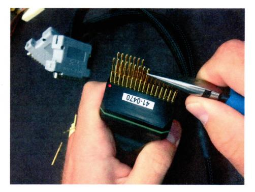
c) Pull straight up on the pin away from the UTI with the pliers.
